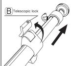
Unlock Band adjust the length of the arm. Once set to the appropriate length, close B to secure.
